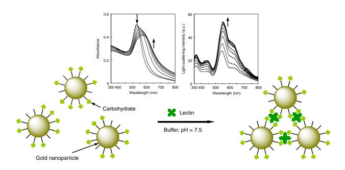
Glycoconjugated gold nanoparticle aggregation was induced by protein—carbohydrate interaction, which shifted the plasmon absorption to longer wavelengths and increased the intensity of plasmon light scattering.
