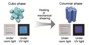
A liquid-crystalline 1,5-naphtharene derivative having dendritic moieties and amide groups has been prepared. The mechanical and thermal stimuli induce the phase transition of this compound from the cubic phase to the columnar phase, leading to the luminescent colour change from light blue to blue. This material is colourless due to little absorption in the visible region.
